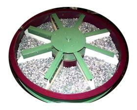
Rotating Carousel Divider Option allows parts to be finished without part to part contact. The number of removable dividers is determined by your production rate. Nylon dividers can be removed to adjust spacing for larger parts. Carousel rotates on the heavy duty center bearing.
