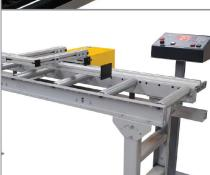
The PMI-Go2 PD-50 is an auto go-to stop placed on the saw's outfeed (exit) side. The operator simply enters a dimension into the keypad control, and the stop automatically moves to the programmed dimension.
