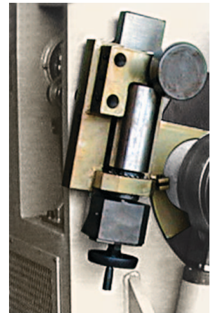
Tri-directional lateral material guides standard Tri-directional hydraulic powered: 308 - 315
