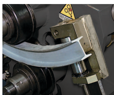
Standard rolls used to roll junior I beams EZ and Hard way
