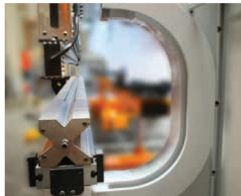
■ Up to 1500 mm special throat depth is offered for wide bendings (O)
