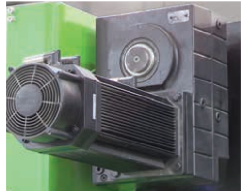
■ Top beam is moved with high efficient synchronous ac servo motors (S)
