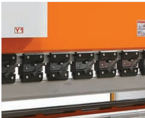
■ Promecam type top tool clamping system which can be manually installed and removed easily (S)
