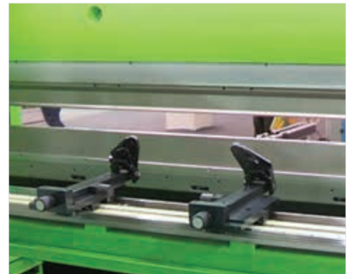
■ 4 axes (X, R, Z1, Z2) Backgauge with servo motor Backgauge with positioning accuracy of 0.05 mm according to the desired geometry (S)
