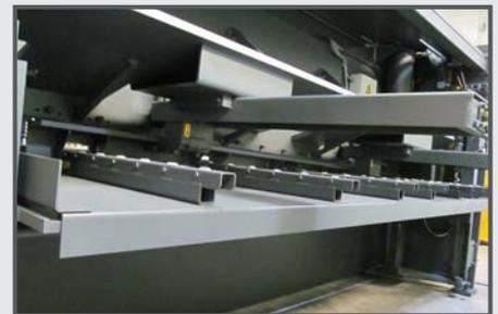
**PNEUMATIC SHEET SUPPORT SYSTEM**, scrap chute and scrap container, counter rolls, alignment cylinders and stacker with automatic adjustable arms.
